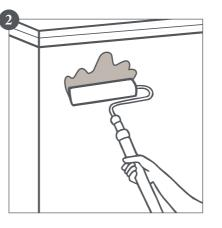
Step 2: Apply the wallpaper paste to the wall Apply the paste-the-wall wallpaper paste to the wall with a paste brush or roller, pasting beyond the plumb line (drawn with the aid of a spirit level). This will allow you to reposition the drop if you need to make any adjustments or straighten up the drop.
