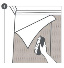
Step 4: Paste and repeat Continue to paste the wall section by section and hang each drop from top to bottom according to the pattern match repeat. Each drop should be hung with a butted seam so that each edge is touching the next but not overlapping. Ensure that any excess paste is gently wiped from the surface of the paper before it dries.
